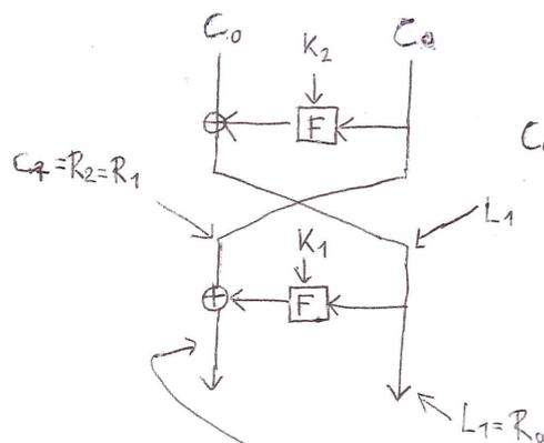
$$C_0 \oplus F(k_2, C_1) = L_1 \oplus F(k_2, R_1) \oplus F(k_2, R_1) = L_1$$
