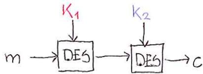
$$c = \text{DES}_{K_1}(\text{DES}_{K_2}(m))$$
